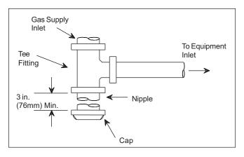
Figure 5. Typical design for a sediment trap/drip leg.
